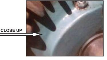
**Test Surface:** Old/Retired Electric Motor left outdoors for many years. When in operation, the motor ran 3-4 months non-stop at a temperature of 140°F.
