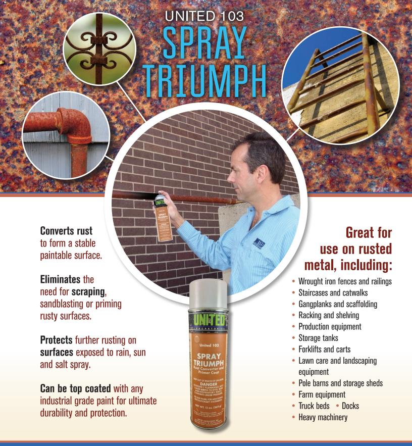
**SPRAY TRIUMPH** is an actual rust converter which quickly and easily converts residual rust to a black protective polymeric coating. This inert protective coating prevents further rusting and corrosion.
